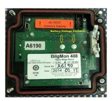
The newer model BilgMon 488 is equipped with a replaceable battery shown on the right below the yellow arrow. As a result, when the battery weakens the unit display will read "Batterylow: 0.5V Replace battery." The battery can then be safely removed because it utilizes a capacitor that ensures enough energy to maintain the stored data for several hours. Click here for the applicable manual.
